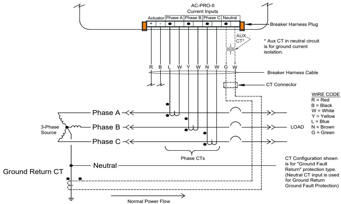
**Figure 5.4: AC-PRO-II Typical Ground Return Wiring Diagram**
