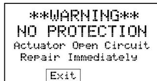
**Figure 20.2: Actuator Open screen**
