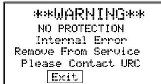
**Figure 20.1: Internal Error Screen**
