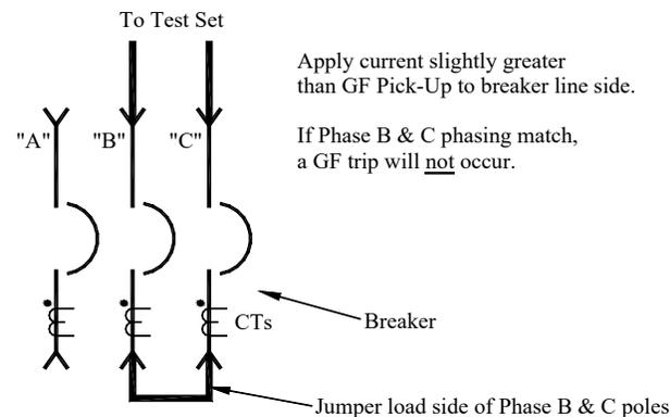
**Figure 14.3: Phase B & C, CT Polarity Test**
