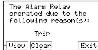
**Figure 20.3: Alarm Screen (example shown is Trip Alarm)**
