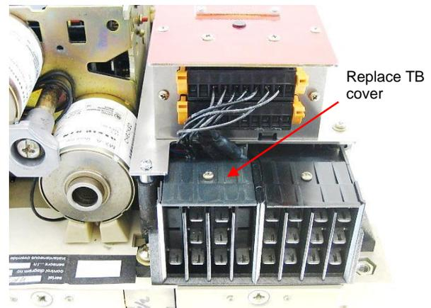
Replace the terminal block cover using the existing screw.
